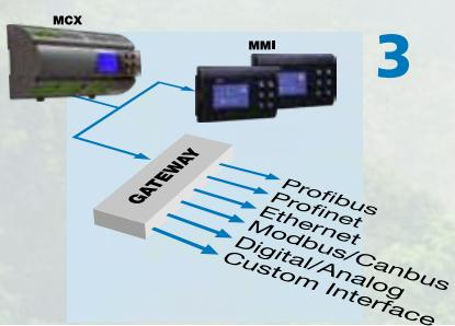
**3** **PLC alphanumeric controller User Friendly** | Automatic management of the zones, available in multiple languages, predisposition for serial connections, description completed of functions and alarms.
